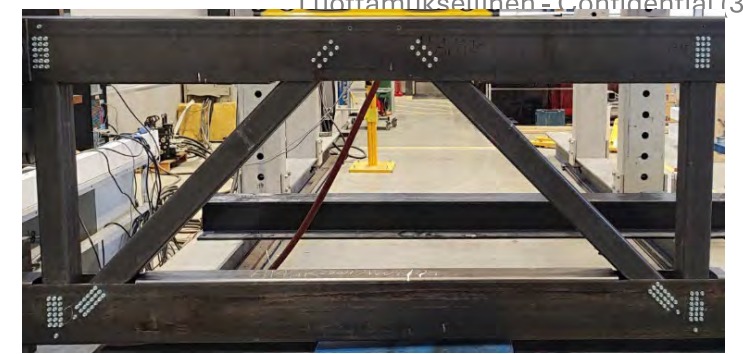
14 K-joint sub-truss tests and 12 FEAs
